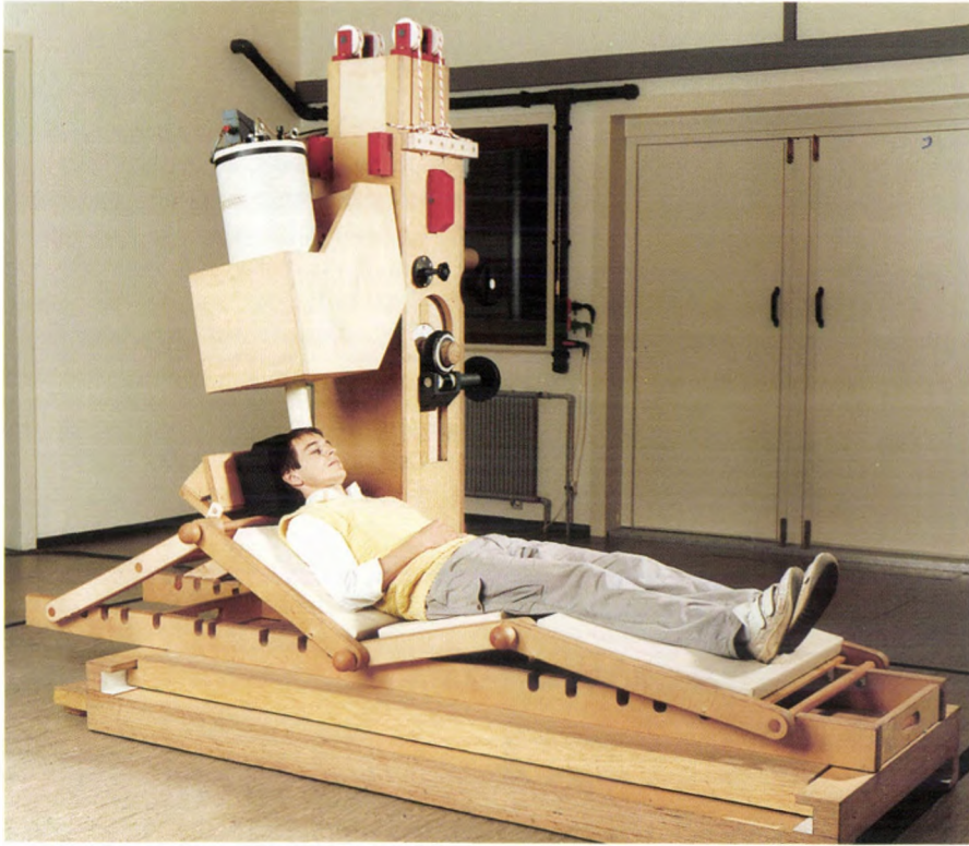
Fig. 11. The SQUID configuration at the Hamburg laboratories. Above the patient's head is the magnetometer, and above that the vessel containing liquid helium. The frame and the patient table are made entirely of non-ferromagnetic material.
