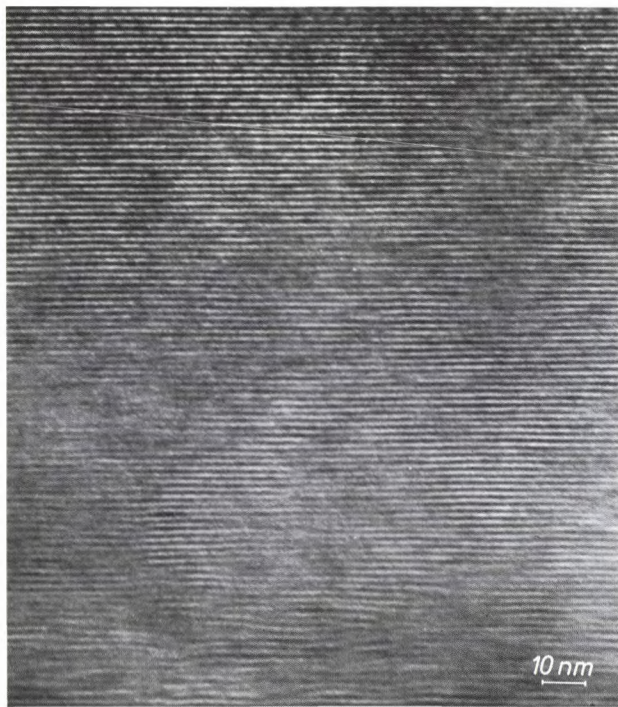
Fig. 2. Cross-sectional (002) dark-field micrograph, obtained by transmission electron microscopy, of a superlattice grown by molecular beam epitaxy. The superlattice comprises 100 periods of alternate layers of AlAs and GaAs, each three monolayers thick. The micrograph was taken by J. P. Gowers at PRL.
