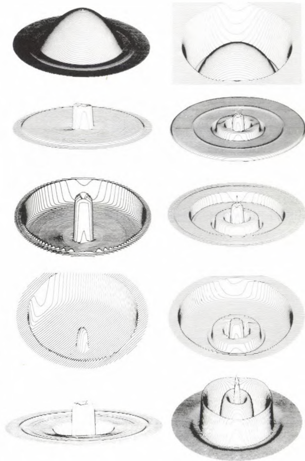
Fig. 10. Various measured 3-dimensional index profiles in the preforms used in the drawing process. The radial scales are not the same in all the diagrams. The diagram at the lower right corresponds to the DFSM fibre (profile C in fig. 5). When fibres are drawn from the preforms the shape of their index profiles is virtually unchanged.
