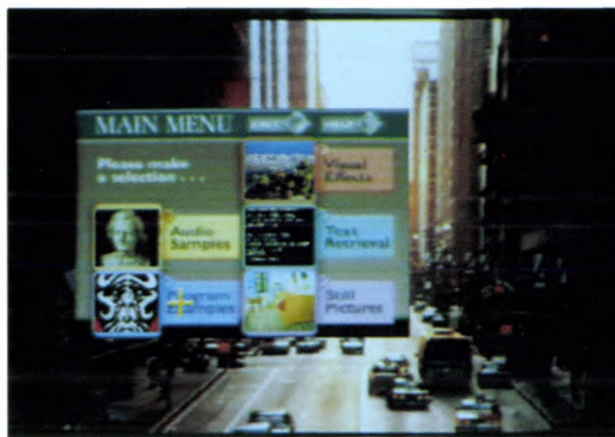
Fig. 6. Another method of combining image planes; see also fig. 4. Image plane 2 is transparent inside the frame, so that image plane 3, which contains the main menu, becomes visible. Image plane 1 contains the cursor.
