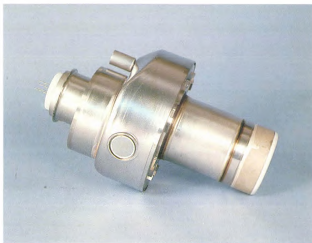
Fig. 1. The new Philips MRC200 diagnostic X-ray tube with an anode mounted in spiral-groove bearings lubricated by liquid metal. The anode diameter is 200 mm. The rated input is 85 kW [7] .
